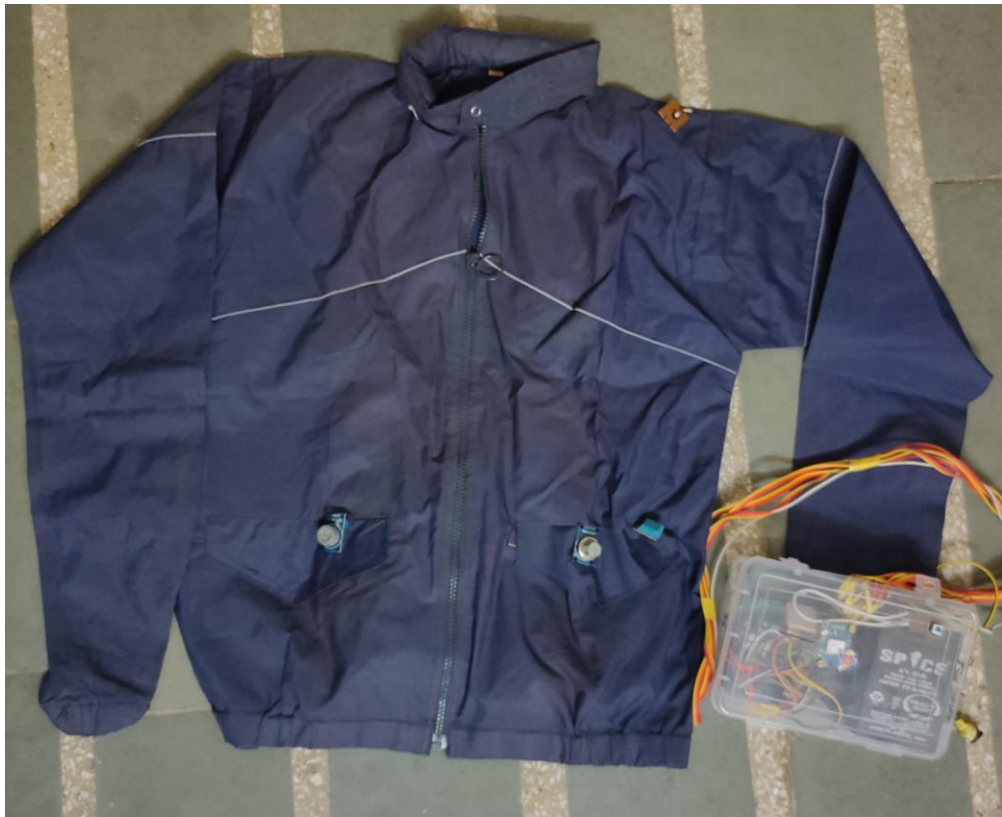
Figure 4.6 Prototype of Jacket and Sensor mounted on it
