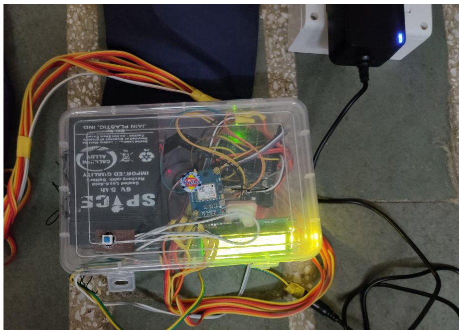
Figure 4.9 Prototype of Power box and Sensor and Microcontroller mounted on it with Applied voltage
