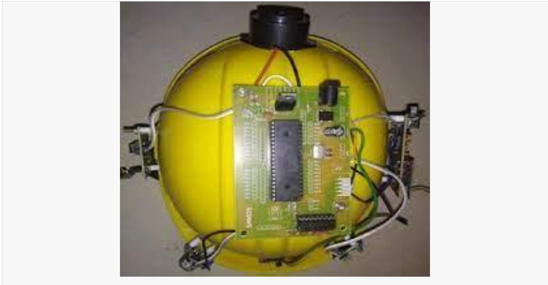
Figure 2.5 Helmet with sensors
