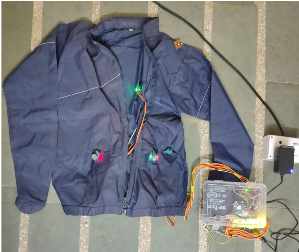
Figure 4.8 Prototype of Jacket and Sensor mounted on it with Applied voltage
